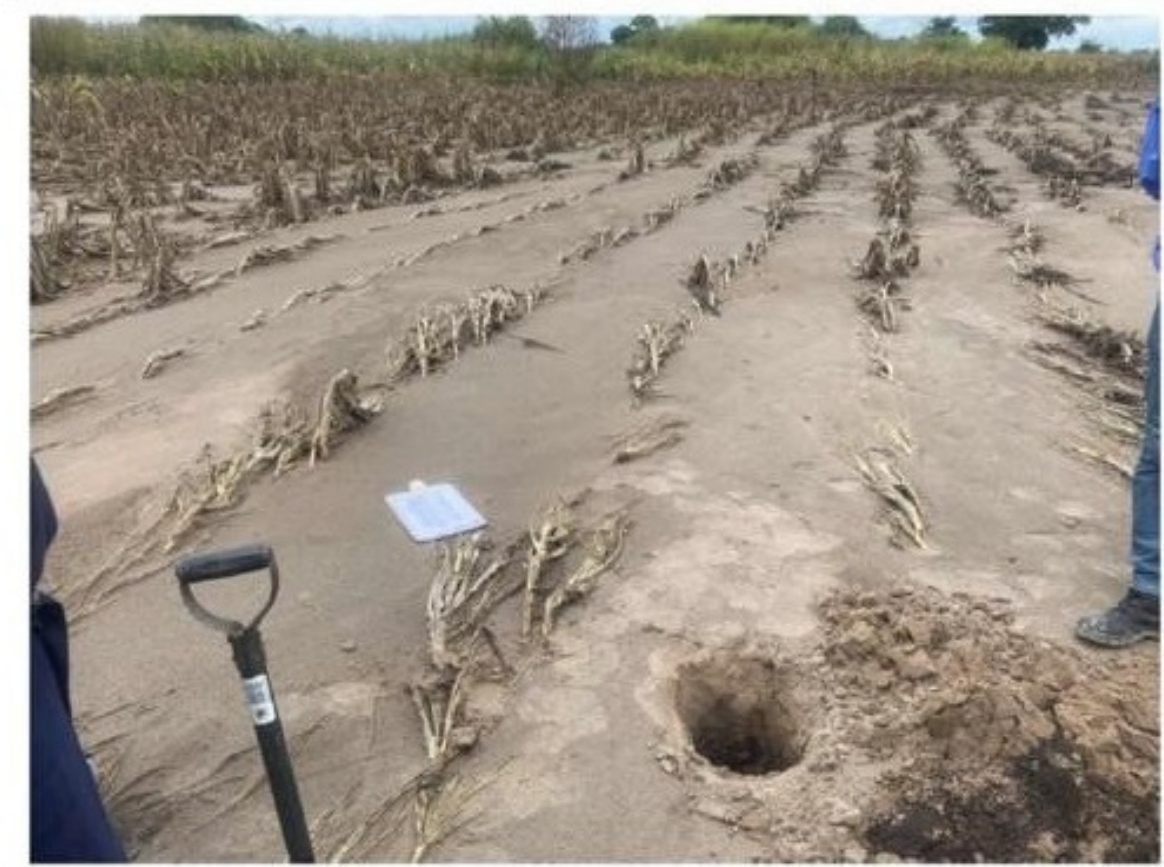
Thickness of tailings deposited in the maize field in the inhabited area in the Chambishi.
